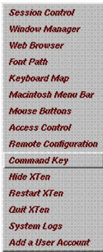
**X Meta and Alt Keys.** Under X<sup>Ten</sup>, the Macintosh <Command> key functions by default as an “X Meta” (or when shifted, “Alt”) key. Many applications, including the Motif Window Manager, use the Meta and Alt keys as keyboard modifiers. Use the configuration manager to change the default operation of the <Command> key to Alt (or when shifted, Meta).
