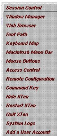
X<sup>Ten</sup> can be configured to control X sessions using either the *Xinit* program or XDM. *Xinit* provides the simplest level of control. It manages a single X session and doesn't require user authentication. XDM can manage a collection of either local or remote X displays. Under XDM, users are presented with a uniform entry into the X Window system. User authentication is required.
